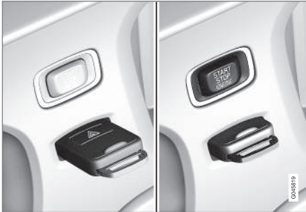
Ignition switch with remote control key extracted/inserted.
