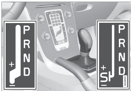
D: Automatic gear positions. +/-: Manual gear positions. S: Sport mode*. 4
