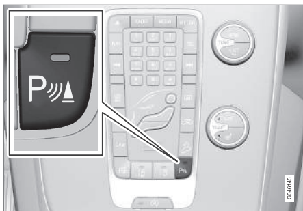
On/Off for the sensors for parking assistance and CTA 30 .
