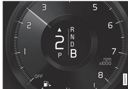
Gear shift indicator in the driver display 2 .
