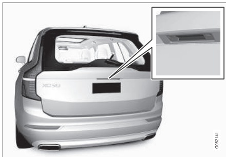
Rubber plate with pressure-sensitive surface.
