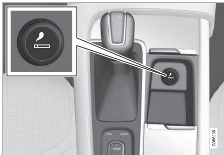
Cigarette lighter in the tunnel console, front seat.
