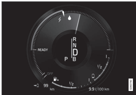
The electric motor cannot supply the amount of engine power requested and the internal combustion engine starts.
