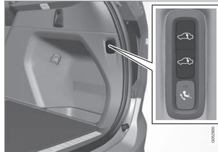
Controls for raising/lowering the car's rear section.
