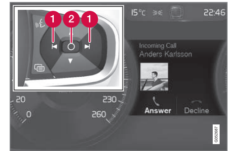
Message in the driver display and the steering wheel's right-hand keypad.
