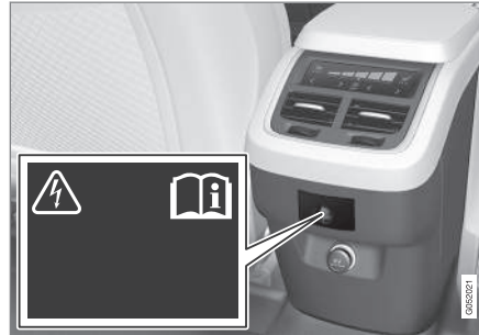
230 V electrical socket in tunnel console, second seat row.
