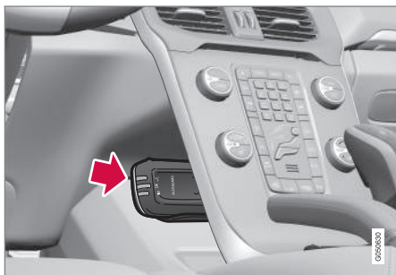
Handheld unit storage and charging station.
