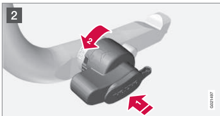
2 Push in the locking wheel and turn it anticlockwise until you hear a click.
