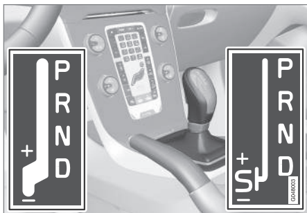
D: Automatic gear positions. +/–: Manual gear positions. S: Sport mode 7 .
