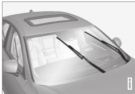
Viskerblader i servicestilling.
