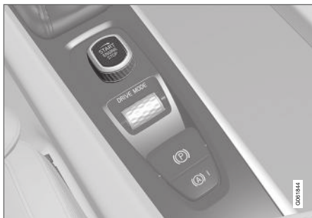
Start knob in the tunnel console.
