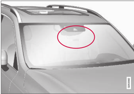
Location of the camera unit.
