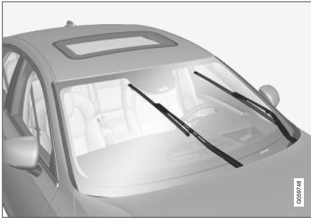
Viskerblader i servicestilling.
