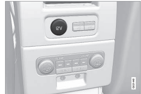
12 V socket in tunnel console, rear seat.
