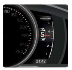
When using the Geartronic manual shifting mode, a white arrow will appear above or below the number of the current gear to prompt the driver to shift up or down (digital instrument panel\* shown).
