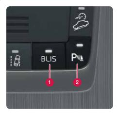
**Blind Spot Information System (BLIS)** indicates the presence of a fast approaching vehicle or a passing vehicle in the door mirror's blind area.
