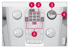
Centre console, controls for radio functions.
