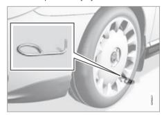
Screw together the towing eye with the wheel wrench\* until the stop position as shown in the following illustration.
