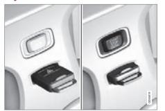
Ignition switch with remote control key extracted/inserted
