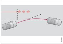
LKA steers and warns with pulsing steering wheel vibrations<sup>1</sup>.
