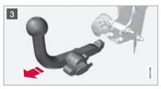
Turn the locking wheel down fully, until it comes to a stop. Hold it in this position while pulling the towball rearward and upward.
