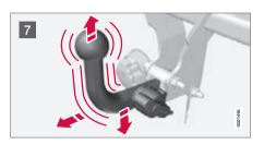
7 Check that the towball section is secure by pulling it up, down and back.
