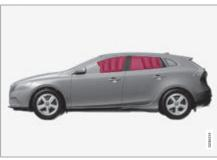
The inflatable curtain (IC) is a part of the SIPS system. It is fitted in the headlining along both sides of the roof and protects the car's occupants sitting in the outer seats. A sufficiently violent collision trips the sensors and the inflatable curtain is inflated. The inflatable curtain helps to prevent the driver and passengers from striking their heads on the inside of the car during a collision.
