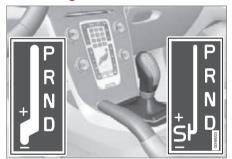
**D**: Automatic gear positions. +/-: Manual gear positions. **S**: Sport mode\*.1
