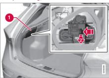
Direction indicators, brake lights and rear lights are replaced from inside the cargo area.
