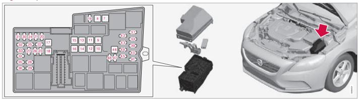
On the inside of the cover there are tweezers that facilitate the procedure for the removal and fitting of fuses.
