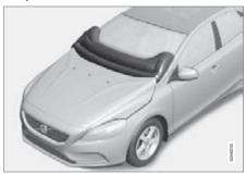
The airbag (Pedestrian Airbag) is fitted under the bonnet near the windscreen. In the event of a frontal collision with a pedestrian, the sensors in the front bumper react and the airbag inflates if required based on the force of the impact. The sensors are active at a speed of approx. 20-50 km/h and an ambient temperature between -20 and +70°C.
