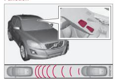
Laser sensor transmitter and receiver window1.
