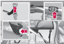
The cargo net can be easily removed and folded up.
