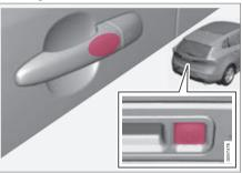
Cars with the Keyless-drive system have a touchsensitive area on the outer handle of the doors and a rubberised button next to the tailgate's rubberised pressure plate.
