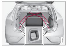
The load retaining eyelets are used to fasten straps in order to anchor items in the cargo area.
