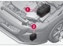
(1) Starter battery<sup>3</sup> (2) Support battery
