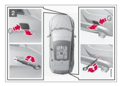
Take out the towing eye that is located under the floor hatch in the cargo area.
