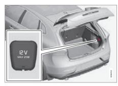
Lower the cover to access the electrical socket.
