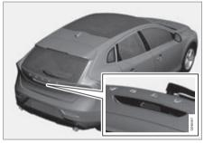
Rubber plate with electrical contact.
