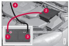
If the battery is flat then the car can be started with current from another battery.
