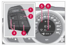
The steering wheel buttons and combined instrument panel in cars **without** speed limiter<sup>1</sup>.
