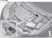
The fluid reservoir is located on the driver's side.
