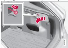
The fuel filler flap can be opened manually when it cannot be opened from outside.
