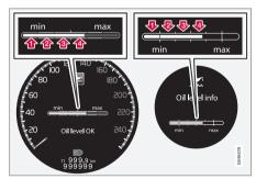
The figures 1-4 represent filling level. Do not fill more oil if filling level (3) or (4) is shown. The recommended filling level is 4. Message and graph in the display. The left-hand display shows the
