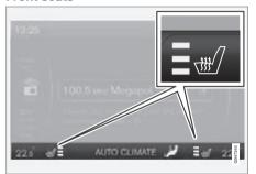
Current heat level is shown in the centre console display screen.
