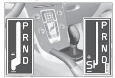
**D**: Automatic gear positions. +/-: Manual gear positions. **S**: Sport mode\*.<sup>3</sup>
