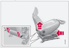
The passenger seat backrest can be folded forward to make room for long loads.
