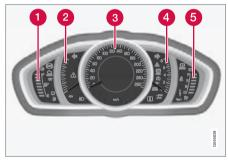
Fuel gauge. When the indicator lowers to only one white marking<sup>1</sup>, the yellow indicator symbol for low level in the fuel tank
