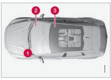
Fuse box locations in a left-hand drive car. In a right-hand drive car the fuse box under the glovebox changes sides.
