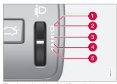
Thumbwheel positions for different load cases.
