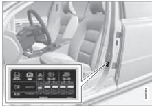
The tyre pressure decal on the driver's side door pillar (between frame and rear door) shows which pressures the tyres should have at different loads and speed conditions. This is also specified in the tyre pressure table, see page 393.
