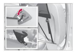
Hook the cargo net's anchoring straps into the eyes on the rear of the seat slide rails - it is easier if the backrests are straightened and the seats are moved forward slightly.
