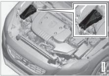
When topping up the coolant, follow the instructions on the packaging. It is important that the mixture of coolant concentrate and water is correct for the prevailing weather conditions. Never top up with water only. The risk of freezing increases with both too little and too much coolant concentrate.
