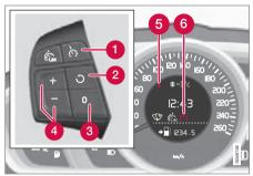
The steering wheel buttons and combined instrument panel in cars **with** speed limiter<sup>1</sup>.
