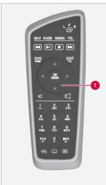
The remote control can be used for all functions in the infotainment system. The remote control's buttons have the same functions as the buttons in the centre console or steering wheel keypad\*.
