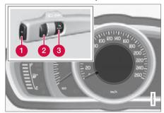
Information display (analogue combined instrument panel) and controls for menu navigation.
