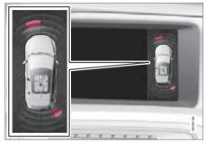
Screen view - showing an obstacle left front and right rear.
