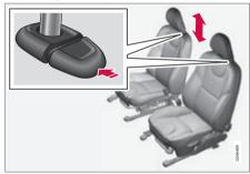
The height of the front seat head restraints can be adjusted.
