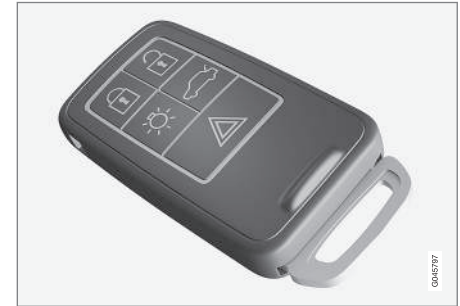
Remote control key in basic version.
