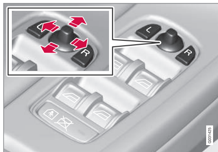
Controls for door mirrors.
