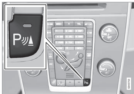
On/Off for parking assistance and CTA sensors.
