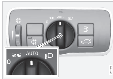
Knob for headlamp control in AUTO position.
