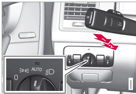
Stalk switch and knob for headlamp control.
