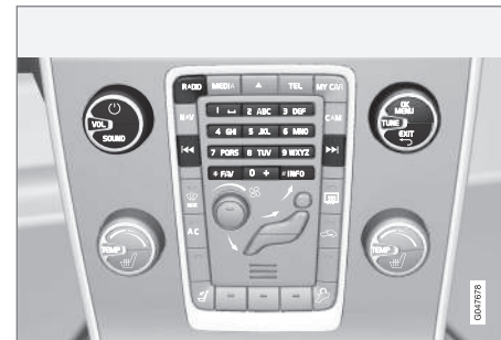
Controls for radio functions.
