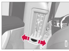
The air vent's thumbwheel<sup>2</sup>.
