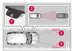
The camera and radar unit measures the distance to the vehicle ahead and detects side markings<sup>55</sup>.
