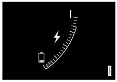
The symbol f is shown in the hybrid battery gauge when Charge is activated.
