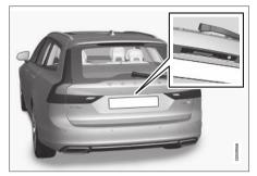
Rubberised pressure plate on the tailgate used for unlocking only.
