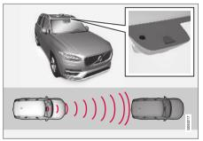
The camera and radar unit measures the distance to the vehicle ahead<sup>37</sup>.
