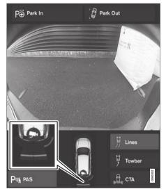
The screen can show coloured sensor fields on the car symbol <sup>118</sup>.
