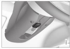
Lever for steering wheel adjustment.
