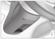
Lever for steering wheel adjustment.
