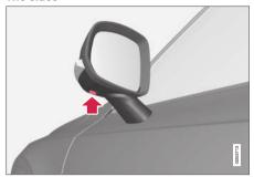
The side cameras<sup>116</sup> are positioned in each door mirror.
