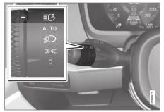
Active main beam is activated with the rotating ring on the stalk switch in position  $\mbox{AUTO}$  .
