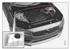
Coolant expansion tank, left-hand drive car.
