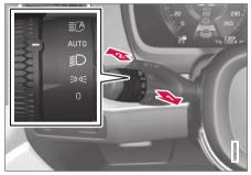
Steering wheel stalk switch with rotating ring.
