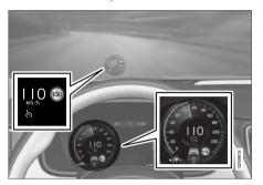
The previous illustration<sup>62</sup> shows that Pilot Assist is set to maintain 110 km/h (68 mph) and that there is no vehicle ahead to follow.
