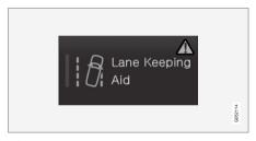
When a warning triangle is shown in the righthand section of the button there is something not working as intended.
