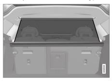
For reasons of safety, the safety net must always be fastened and anchored as described below.
