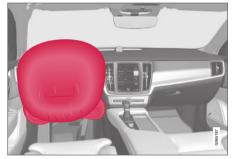
Steering wheel airbag and knee airbag<sup>1</sup> on the driver's side in the front seat.
