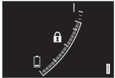
The symbol **1** is shown in the hybrid battery gauge when Hold is activated.
