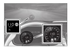
The previous illustration<sup>54</sup> shows that the adaptive cruise control is set to maintain 110 km/h (68 mph) and that there is no vehicle ahead to follow.
