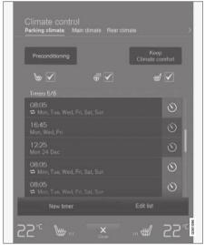
Functions belonging to the parking climate control are controlled from the **Parking climate** in climate view in the centre display.
