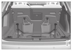
There are two bag hooks and an elastic strap<sup>3</sup> in the cover, which is part of the floor hatch in the cargo area. The strap can be fitted in four different positions.
