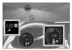
The previous illustration<sup>54</sup> shows that the adaptive cruise control is set to maintain 110 km/h (68 mph) and at the same time is following a vehicle ahead which is keeping the same speed.
