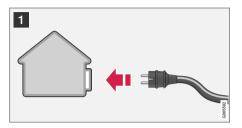
Connect the charging cable to a 230 V socket. Never use an extension cable.
