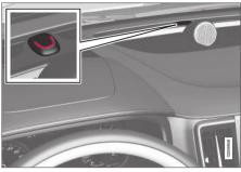
The lock and alarm indicator on the instrument panel show the status of the alarm system.
