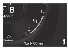
The energy in the hybrid battery is used for the electric motor, but also to cool or heat the car. The trip computer calculates an approximate distance for the energy left in the hybrid battery.
