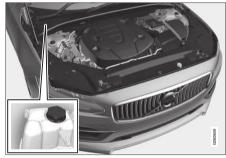
Coolant expansion tank, right-hand drive car.
