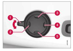
Activate the multi-function control by turning the control 1 upwards/downwards. The seat settings view will be shown in the centre display.
