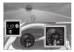
The previous illustration <sup>62</sup> shows that Pilot Assist is set to maintain 110 km/h (68 mph) and at the same time is following a vehicle ahead which is keeping the same speed.
