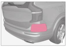
Keep the surface indicated clean – on both the left and right-hand sides of the car<sup>78</sup>.
