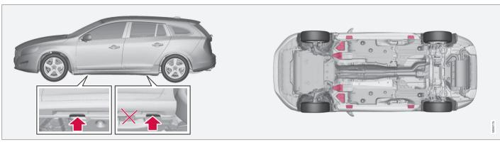
Jacking points (arrows) for the jack that belongs to the car and lifting points (marked in red).
