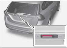
Rubber plate with electrical contact.
