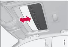
One long press on the lock button closes the sunroof and all the windows, see Remote control key - functions (p. 166) and Locking/unlocking - from the inside (p. 179). The doors and the tailgate are locked. To interrupt closing, press the lock button again.
