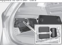
The emergency puncture repair kit is located behind the side hatch in the cargo area.
