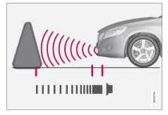
The distance covered in front of the car is about 0.8 metres. The acoustic signal for obstacles in front comes from one of the front loudspeakers.
