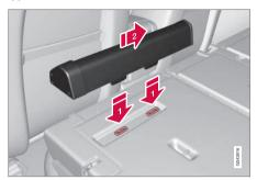
The two-part safety net cassette is secured on the rear of the backrest. The narrowest cassette is secured on the left-hand side (seen from the tailgate).
