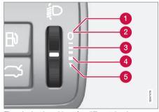
Thumbwheel positions for different load cases.
