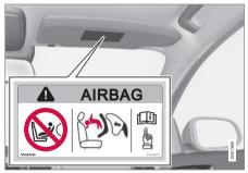
Alternative 1: Position of airbag label on passenger side sun visor.
