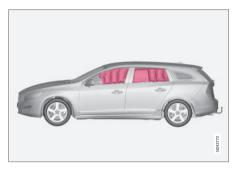
Inflatable curtain IC (Inflatable Curtain) is part of the SIPS system (p. 36) and the airbag system (p. 32). It is fitted along both sides of the headlining and helps protect the driver and passengers in the car's outer seats. A sufficiently violent collision trips the sensors and the inflatable curtain is inflated.
