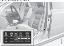
The tyre pressure label on the driver's side door pillar (between frame and rear door) shows which pressures the tyres should have at different loads and speed conditions. This is also specified in the tyre pressure table, see Tyres - approved tyre pressures (p. 435).
