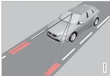
(The figure is schematic - not model specific.) A camera reads the side lines of the road/ lane
