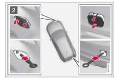
Take out the towing eye that is located under the floor hatch in the cargo area.
