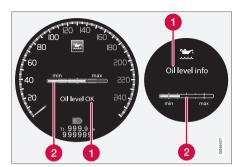
Message and graphic in the display. The lefthand display is shown in the digital combined instrument panel and the right-hand in the analoaue.
