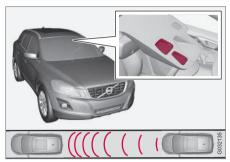
Laser sensor transmitter and receiver window14.
