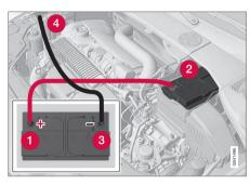
When jump starting the car, the following steps are recommended to avoid short circuits or other damage:
