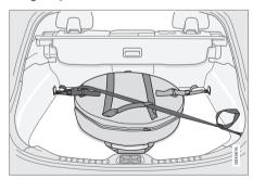
Cars with four load retaining eyelets.
