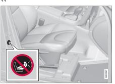
Alternative 2: Position of airbag label on passenger side door pillar. The label becomes visible when the passenger door is opened.
