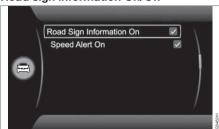
The combined instrument panel's speed symbol display can be disabled. The function can be activated/deactivated in the menu system **MY CAR**. For a description of the menu system, see MY CAR (p. 114).
