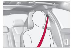
Correctly fitted seatbelt.
