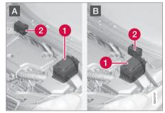
A: Left-hand drive car. B: Right-hand drive car. (1) Starter battery<sup>17</sup> (2) Support battery.
