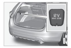
Lower the cover to access the electrical socket.
