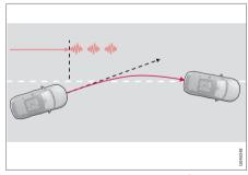
Warning with steering wheel vibration<sup>24</sup>.
