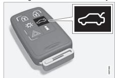
The alarm for the tailgate can be disarmed\* and the tailgate unlocked on its own by using the remote control key's button.
