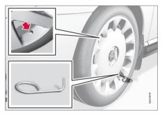
Screw together the towing eye with the wheel wrench\* to the stop position.
