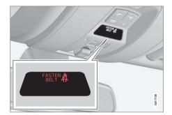
The audio reminder is speed dependent, and in some cases time dependent. The visual reminder is located in the roof console and in the combined instrument panel (p. 65).
