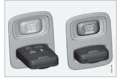
Ignition switch with remote control key extracted/inserted.
