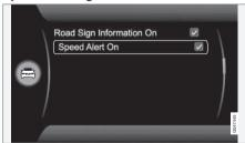
The driver can opt to receive a warning when the applicable speed limit is exceeded by 5 km/h or more. This warning is given by the symbol showing the applicable maximum speed temporarily flashing when this speed is exceeded. The function can be activated/ deactivated in the menu system **MY CAR**. For a description of the menu system, see MY CAR (p. 114).
