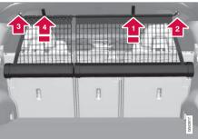
Pull the net up from the cassettes. The net is self-locking after approx. one minute if the rear seat's backrests are raised.
