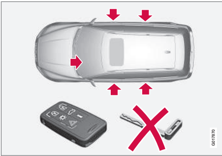
Locking/unlocking points with private locking activated.
