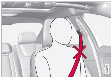
Incorrect height adjustment
