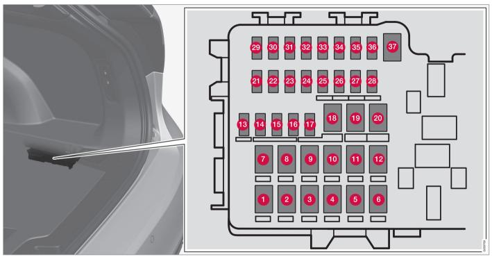
The central electrical unit is located on the right-hand side.
