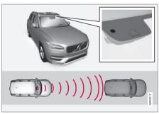
The camera and radar unit measures the distance to the vehicle ahead<sup>5</sup>.
