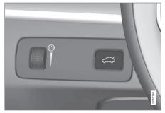
Opening/closing button on the instrument panel.
