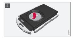
The battery (+) side is facing upwards. Then carefully prize loose the battery as illustrated.
