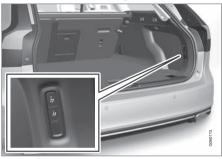
If the car is equipped with electronic folding of the rear seat\* there are buttons located in the cargo area. The backrests can also be lowered manually.
