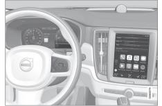
The app menu in the driver display can be used instead of using the centre display.
