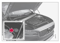
Filling of washer fluid takes place in the reservoir with a blue cap.
