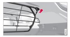
3. Position the safety grille's brackets on the roof mountings.
