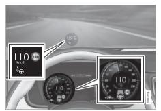
The previous illustration<sup>11</sup> shows that Pilot Assist is set to maintain 110 km/h and that there is no vehicle ahead to follow.
