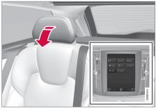
The outer head restraints can be lowered in two ways via the centre display:
