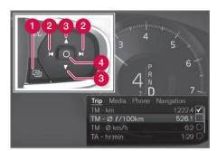
Open and navigate in the app menu<sup>35</sup> using the righthand steering wheel keypad.
