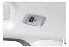
Reading lamp above the rear seat in cars with panorama roof\*.
