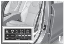
The tyre pressure label on the driver's side door pillar (between frame and rear door) shows which
