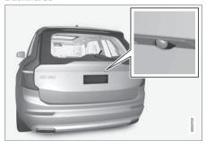
The backwards-facing camera  $\!\!^{27}$  is fitted above the registration plate.
