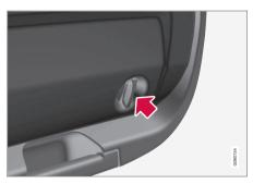
Detach the panel on the inside of the tailgate by first turning the two knobs a quarter turn anticlockwise and then unhooking the panel. Place the panel to one side.
