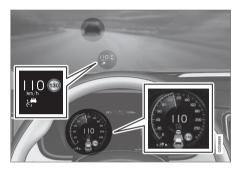
The previous illustration<sup>8</sup> shows that the adaptive cruise control is set to maintain 110 km/h and at the same time follow the vehicle ahead that is keeping the same speed.
