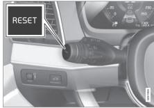
Reset the trip meter TM with one long press on the **RESET** button on the left-hand stalk switch.
