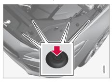
Press down the pins into the plastic cover's four clips using a screwdriver or similar and lift away the cover.
