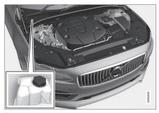
Coolant expansion tank, right-hand drive car.
