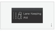
The function is deactivated when the LED indicator is extinguished.
