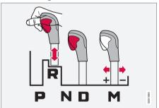
The gear selector can be moved forward and back freely between  $\bf N$  and  $\bf D$ . Other positions are locked with a latch that is released with the inhibitor button on the gear selector.
