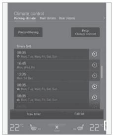
Preconditioning and climate comfort retention are controlled from the **Parking climate** tab in the centre display's climate view.
