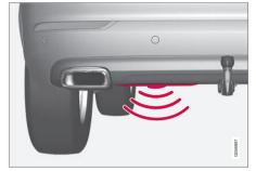
The sensor is positioned to the left of centre in the bumper<sup>13</sup>.
