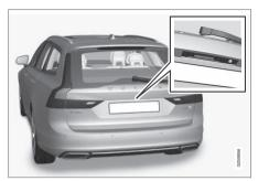
Rubberised pressure plate on the boot lid used for unlocking only.
