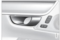
Opening handle for alternative unlocking in the front door.
