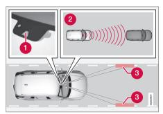
The camera and radar unit measures the distance to the vehicle ahead and detects side markings9.
