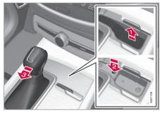
If the car cannot be driven, e.g. due to a discharged battery, the gear selector must be
