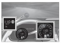
The previous illustration<sup>8</sup> shows that the adaptive cruise control is set to maintain 110 km/h and that there is no vehicle ahead to follow.
