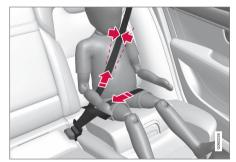
Correct position, the seatbelt must pass over the shoulder
