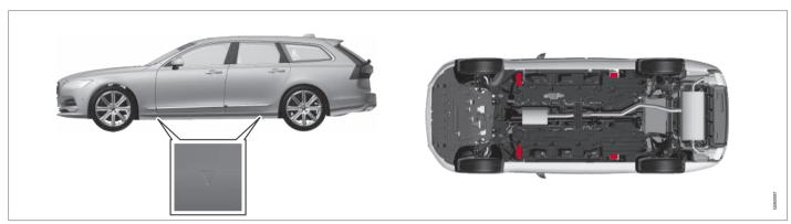
The triangles in the plastic cover indicate the locations of the lifting points (marked in red).
