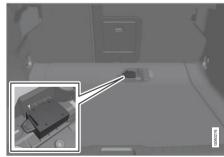
Fit a personal SIM card into the holder under the cargo area floor.
