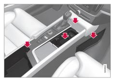
Storage spaces with cup holder, ashtray\*, electrical socket and cigarette lighter\*, mesh pocket\*, as well as an AUX/USB socket in the tunnel console.
