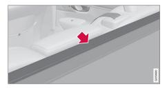
Fold the cargo cover's front sealing disc forward to eliminate the space between the cargo cover and the rear seat's backrests.
