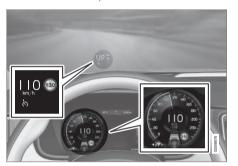
The previous illustration<sup>11</sup> shows that Pilot Assist is set to maintain 110 km/h and that there is no vehicle ahead to follow.
