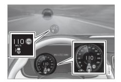
The previous illustration <sup>11</sup> shows that Pilot Assist is set to maintain 110 km/h and at the same time follow the vehicle ahead that is keeping the same speed.
