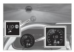
The previous illustration<sup>11</sup> shows that Pilot Assist is set to maintain 110 km/h and at the same time follow the vehicle ahead that is keeping the same speed.
