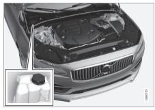
Coolant expansion tank, left-hand drive car.
