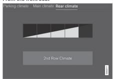
The fan control buttons in the tab **Rear climate** in the climate view.
