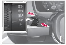
Steering wheel stalk switch with rotating ring.
