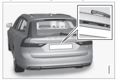
Rubber plate with pressure-sensitive surface.
