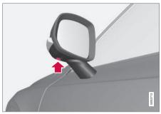
The side cameras<sup>27</sup> are positioned in each door mirror.
