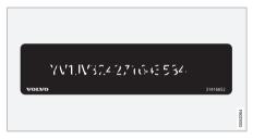
**7** Decal for the car's identification number - VIN (Vehicle Identification Number).
