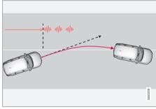
Lane assistance warns with steering wheel vibrations<sup>23</sup>.
