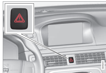
Button for hazard warning flashers.
