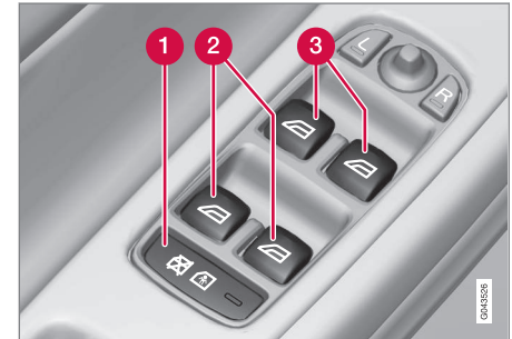
Driver's door control panel.
