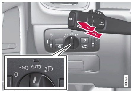
Stalk switch and knob for headlamp control.
