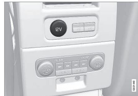
12 V socket in tunnel console, rear seat.
