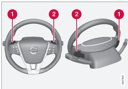
Steering-wheel mounted gear shift paddles
