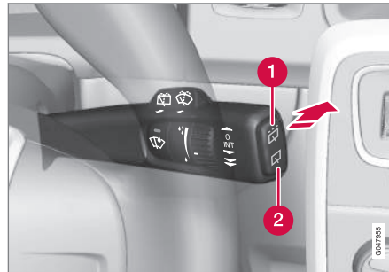
Move the lever forward to start the tailgate washer.
