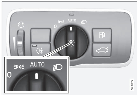
Headlight switch in the AUTO position
