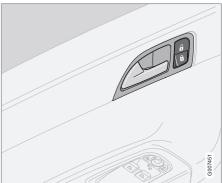
With the central locking button on the driver's door, the doors and tailgate can be locked or unlocked simultaneously.
