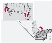
The passenger seat backrest can be folded forward to make room for long loads.
