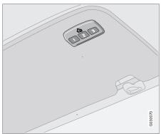
HomeLink® is a programmable remote control which can control up to three different devices (e.g. garage door, alarm system, outdoor lighting and indoor lighting etc.) and in doing so replace their remote controls. HomeLink® is supplied built into the left-hand sun visor.
