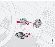
If the alarm cannot be deactivated with the remote control key, e.g. if the key's battery is discharged - the car can be unlocked, disarmed and the engine started as follows:
