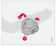
3. Check that the indicator window (3) shows red. If the window does not show red, press in 1 and turn the locking wheel anticlockwise 2 until you hear a click.
