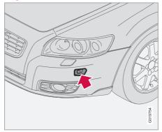
Electrical input to the engine block heater.
