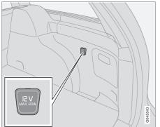
Fold down the cover to access the electrical socket. This socket works regardless of whether or not the ignition is on.
