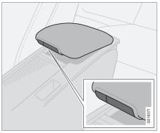
There is a storage space under the armrest. There is also a smaller storage space in the detachable armrest. Press the small button and lift the armrest to open the shallow compartment. Press the large button and lift the armrest to open the deeper compartment.
