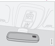
The upper right-hand corner of the rearview mirror has an integrated display that shows the compass direction in which the front of the car is pointing. Eight different directions are shown with English abbreviations: N (north), NE (north east), E (east), SE (south east), S (south), SW (south west), W (west) and NW (north west).
