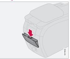
An ashtray is located towards the rear of the tunnel console.
