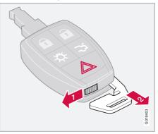
Using the remote control key's detachable key blade:
