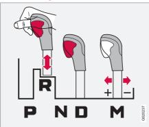
The gear selector can be moved forward and back freely between  ${\bf N}$  and  ${\bf D}$ . Other positions are locked with a latch that is released with the inhibitor button on the gear selector.
