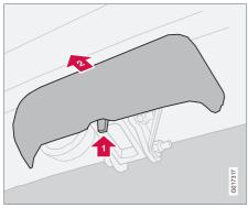
1. Remove the protective cover by first pressing in the catch in and then pulling the cover straight back 2.
