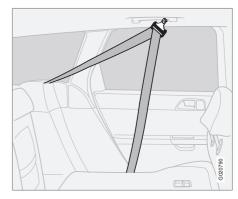
The rear seat backrests can be tipped forwards together, or individually, to make it easier to transport long objects. To avoid damaging the seatbelts when folding the backrests up or down, these should be hooked onto the grab handles.
