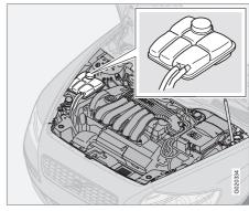
When topping up the coolant, follow the instructions on the packaging. It is important that the mixture of coolant concentrate and water is correct for the prevailing weather conditions. Never top up with water only. The risk
