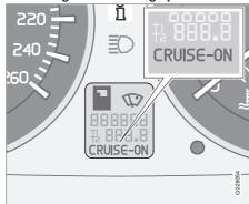
Increase or decrease the speed by pressing and holding + or -. The speed of the car when the button is released is set as the new speed.
