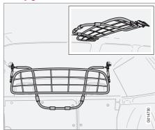
The safety grille is designed to help prevent loads or pets from being thrown forward in the passenger compartment in the event of sudden braking. For safety reasons, the grille must always be correctly fastened and secured.
