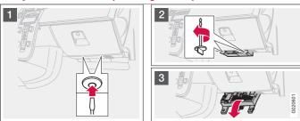
The fuse box has 50 fuse positions. The fuses are located under the glovebox. The box also provides space for several spare fuses. Tools for fuse replacement are located in the relay/fuse box in the engine compartment, see page 242.
