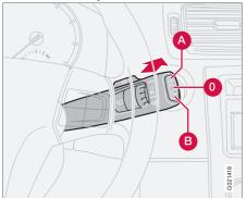
Move the stalk switch forward to start rear window washing and wiping. The wiper blade makes several extra sweeps once washing has finished. The button at the end of the stalk switch has three positions:
