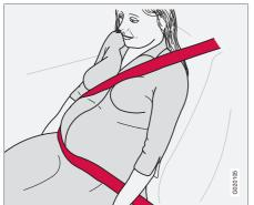
The seatbelt should always be worn during pregnancy. But it is crucial that it be worn in the correct way. The diagonal section of the seatbelt should wrap over the shoulder then be routed between the breasts and to the side of the abdomen.
