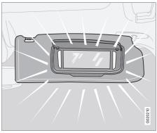
The lamp is automatically switched on and off respectively when the cover is opened or closed.
