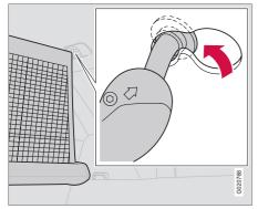
The retractable safety net storage cassette is mounted on the rear of the backrest.
