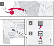
The towing eye is screwed into a threaded socket behind a cover on the right-hand side of the bumper, front or rear.
