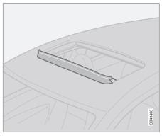
The sunroof has a wind deflector that is folded up when the sunroof is in the open position.
