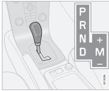
D: Automatic gear positions. M (+/-): Manual gear positions.
