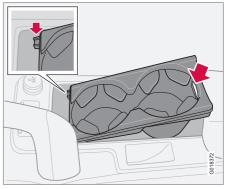
There is space for a double cup holder under the roller cover. The space can be used for storage by lifting out the cup holder. Lift at the rear edge of the cup holder where there is a recess.
