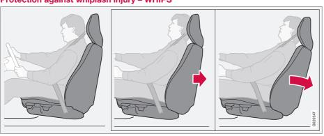
The whiplash protection system (WHIPS) consists of energy absorbing backrests and specially designed head restraints for the front seats. The system is actuated by a rear-end collision, where the angle and speed of the collision, and the nature of the colliding vehicle all have an influence.
