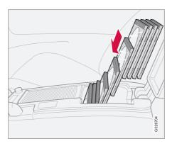
In the deeper compartment there is space for 10 normal CD cases. The cases must be stored vertically on the top edge for all 10 to have space.
