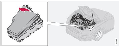
The fuse box has 36 fuse positions. Be sure to replace a blown fuse with a new fuse of the same colour and amperage.
