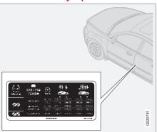
The tyre pressure label on the driver's side door pillar shows which pressures the tyres should have at different load and speed conditions.
