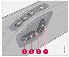
The seats can be adjusted for a certain time after unlocking the door with the remote control key without the key being inserted into the ignition switch. The seat can always be adjusted in key position I or II.
