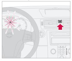
Use the hazard warning flashers (all direction indicators flash) when the car is stopped where it could be a traffic hazard or obstruction. Press the button to activate the function.
