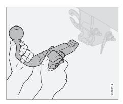
Turn the locking wheel down fully, until it comes to a stop. Hold it in this position while pulling the towbar rearward and upward.
