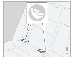
Mounting points for the ISOFIX fixture system are concealed behind the lower section of the rear seat backrest, in the outer seats.
