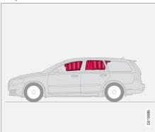
The inflatable curtain IC (Inflatable Curtain) is a part of SIPS and the airbags. It is fitted in the headlining along both sides of the roof and protects the car's occupants sitting in the outer seats. A sufficiently violent collision trips the sensors and the inflatable curtain is inflated. The inflatable curtain helps to prevent the driver and passengers from striking their heads on the inside of the car during a collision.
