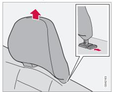
All head restraints can be adjusted vertically to suit the height of the passenger. The upper edge of the head restraint should be aligned with middle of the back of the head. Raise the head restraint as necessary.
