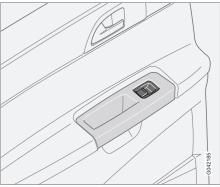
The rear door windows can be operated with the control on each door or with the switch on the driver's door. If the light in the switch for blocking the rear power windows (located in the control panel in the driver's door) is lit, the rear door windows can only be operated from the driver's door. The windows in the rear doors are operated in the same way as the windows in the front doors.
