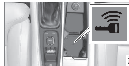
Backup reader's location in the tunnel console.
