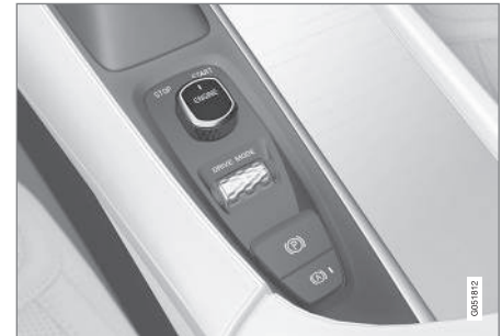
Start knob in the tunnel console.
