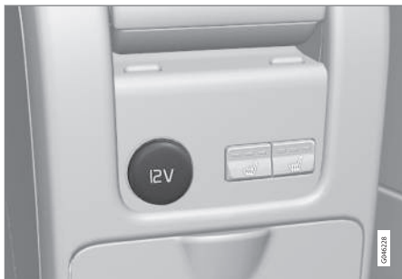
12 V socket in tunnel console, rear seat.
