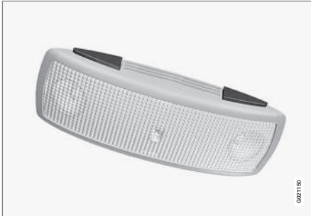
Rear roof lighting.
