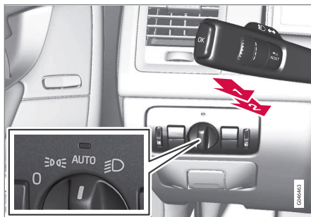
Stalk switch and knob for headlamp control.
