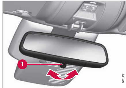
1 Control for dimming
