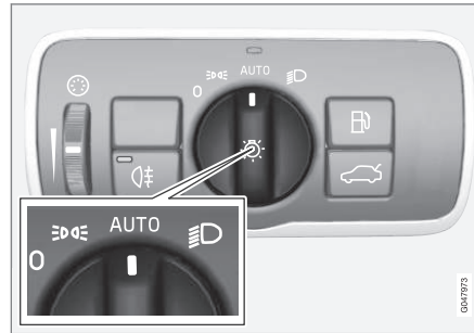
Knob for headlamp control in AUTO position.
