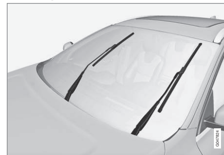
Wiper blades in service position.
