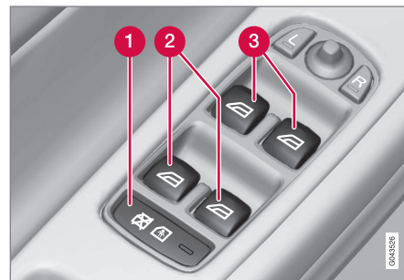
Driver's door control panel.
