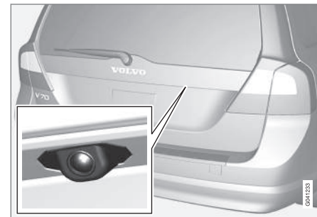
Camera location next to the opening handle.
