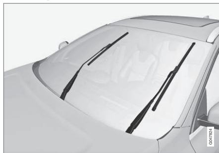
Wiper blades in service position.
