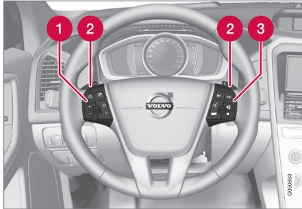
Keypads and paddles in the steering wheel.
