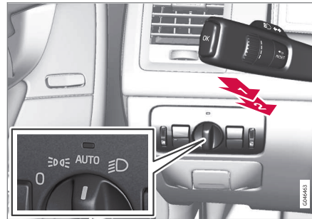
Stalk switch and knob for headlamp control.
