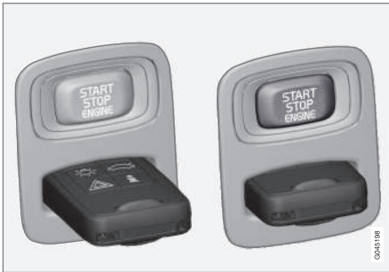
Ignition switch with remote control key extracted/inserted.
