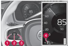
The speed limiter cannot be activated until after the engine has been started. The lowest maximum speed that can be stored is 30 km/h (20 mph).
