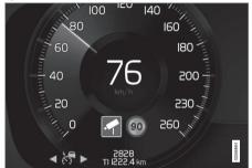
Examples of information on speed camera and speed limit in the driver display.
