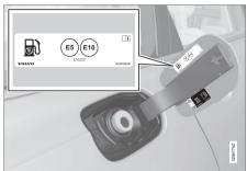
Choose fuel that is approved for use in the car in accordance with the identifier on the inside of the fuel filler flap. See information on approved fuels and the identifier in the sections on "Petrol" and "Diesel" respectively.
