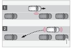
Principle for reversing into parallel parking.
