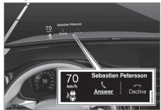
The head-up display shows warnings and information relating to speed, cruise control functions, navigation, etc. in the driver's field of vision. Road Sign Information and incoming phone calls can also be shown in the head up display.
