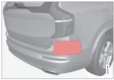
Keep the surface indicated clean – on both the left and right-hand sides of the car<sup>86</sup>.
