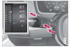
Steering wheel stalk switch with rotating ring.
