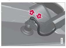
Loosen the washer hose from the bracket.
