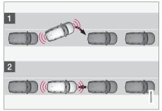
Principle for positioning during parallel parking.
