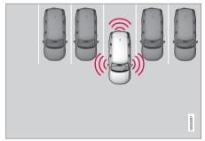
Principle for positioning during perpendicular park-
