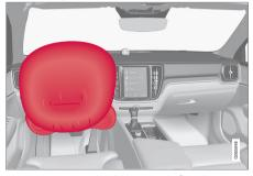
Steering wheel airbag and knee airbag<sup>1</sup> on the driver's side in the front seat.
