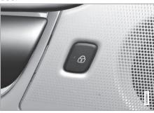
Locking button with indicator lamp in the rear door.
