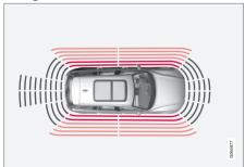
The warning signal pulses intensively at less than approx. 25 cm (0.8 ft) from an obstacle.
