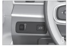
Thumbwheel (to left) for adjusting interior brightness.
