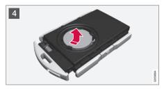
The battery (+) side is facing upwards.
