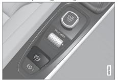
The control for the parking brake is located in the tunnel console between the seats.
