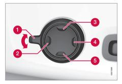
Activate the multi-function control by turning the control upwards/downwards.
