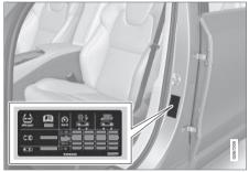
The decal displays the designation for the factory-fitted tyres on the car, as well as load limits and tyre pressure.
