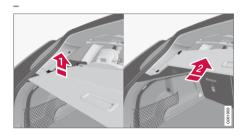
Press the cargo cover's handle section upwards slightly.
