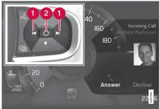
Examples of messages in the driver display  $^{5}$  and the steering wheel's right-hand keypad.
