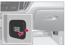
Fit a personal SIM card into the holder by the floor on the passenger side.
