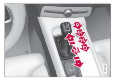
Overview of large gear lever and gear positions.
