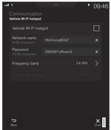
The network operator (SIM card) must support tethering (sharing of the Internet connection).
