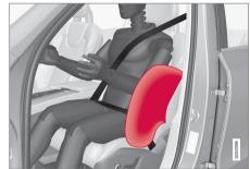
The side airbags are fitted in the outer backrest frames of the front seats and help to protect the driver and passengers in the front seat.
