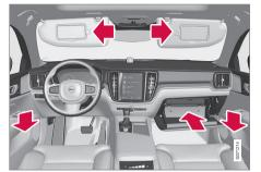
Storage compartment in the door panel, glovebox and sun visor.
