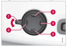
Activate the multi-function control by turning the control 1 upwards/downwards.
