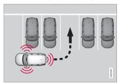
Principle for reversing into perpendicular parking.
