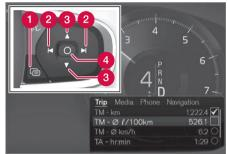
The app menu and the steering wheel's right-hand keypad. The figure is schematic.
