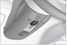
Lever for steering wheel adjustment.
