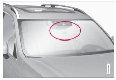
The marked area must be cleaned regularly and kept free from stickers, objects, shade film, etc.
