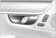
Opening handle for alternative unlocking in the side  ${\tt door^{11}}$ .
