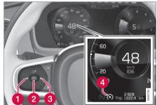
In order to start the cruise control from the standby mode, the car's current speed must be 30 km/h (20 mph) or higher.
