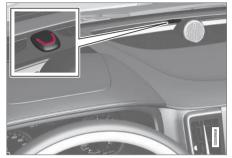
A red LED on the instrument panel flashes once every two seconds when the car is locked and the alarm is armed.
