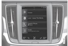
Many of the main functions of the car are controlled from the centre display, a touch screen which reacts to touch. The number of physical buttons and controls in the car is therefore minimal. The screen can even be operated while wearing gloves.
