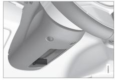
Lever for steering wheel adjustment.
