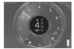
Gear shift indicator in 12-inch driver display for large gear lever\*.
