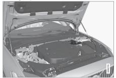
The 12 V support battery is located in the engine compartment.
