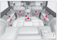
Storage compartment in the door panel, cup holder\* in the centre seat backrest, storage pocket\* on the front seat backrest and also electrical sockets in the tunnel console.
