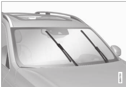
Windshield wipers in the service position.
