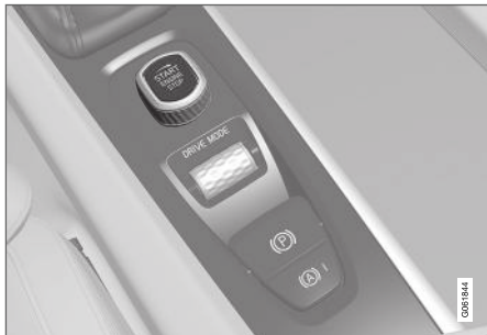
Start knob in the tunnel console.
