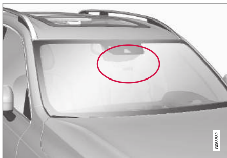
Location of radar sensor.
