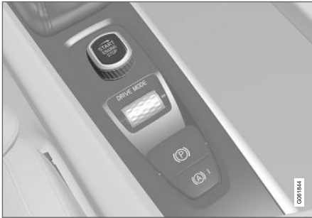
Start knob in the tunnel console.
