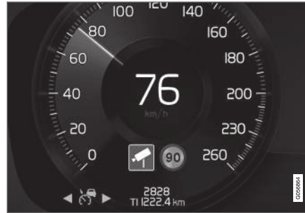
Speed camera information in the instrument panel.
