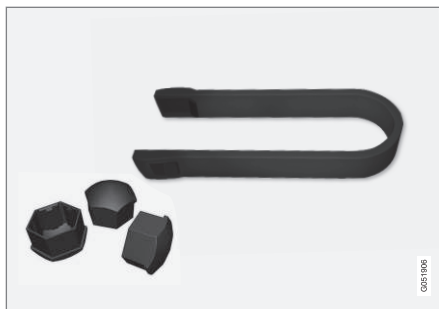
Tool for removing the plastic caps on the wheel bolts.
