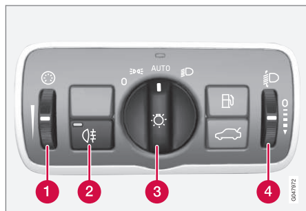
Overview, light switches.
