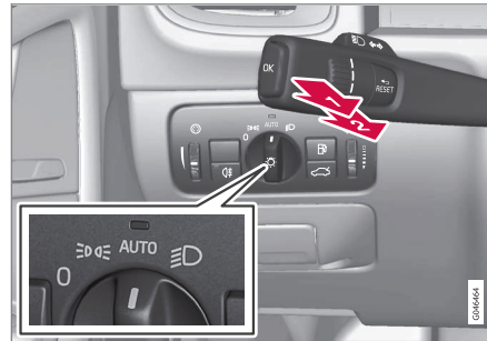
Stalk switch and knob for headlamp control.
