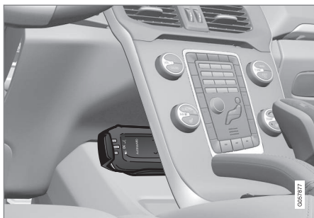
Handheld unit storage location.
