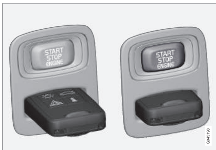
Ignition switch with remote control key extracted/inserted.
