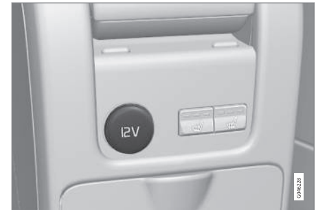
12 V socket in tunnel console, rear seat.
