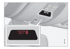
The audio reminder is speed dependent, and in some cases time dependent. The visual reminder is located in the roof console and in the combined instrument panel (p. 55).
