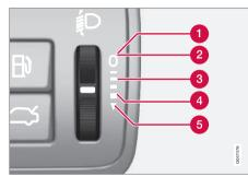
Thumbwheel positions for different load cases.
