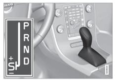
**D**: Automatic gear positions. +/-: Manual gear positions. **S**<sup>8</sup>: Sport mode\*.
