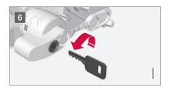
Turn the key anticlockwise to locked position. Remove the key from the lock.
