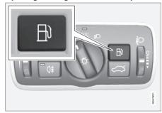
Open the fuel filler flap using the button on the lighting panel - the flap opens when the button is released.
