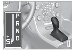
**D**: Automatic gear positions. +S-: Manual gear positions. **S**: Sport mode\*.
