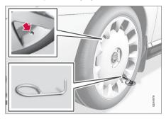
Screw together the towing eye with the wheel wrench\* until the stop position in accordance with the following figure.
