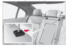
The head restraint can be adjusted vertically to suit the height of the passenger. The upper
