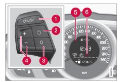
Steering wheel keypad and combined instrument panel.
