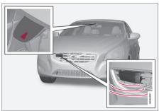
Camera and radar sensor<sup>22</sup>.
