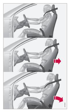
The WHIPS system is actuated by a rear-end collision, where the angle and speed of the collision, and the nature of the colliding vehicle all have an influence.
