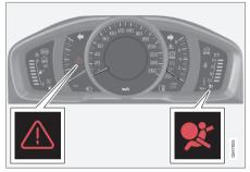
Warning triangle and warning symbol for the airbag system (p. 26) in the analogue combined instrument panel.
