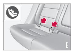
Mounting points for the ISOFIX fixture system are concealed behind the lower section of the rear seat backrest, in the outer seats.
