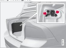
The bulbs in the rear light cluster are replaced from inside the cargo area (not the LED lamps).
