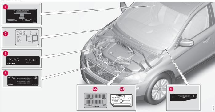
Knowing the car's type designation, vehicle identification and engine numbers can facilitate all contact with an authorised Volvo
