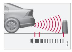
The distance covered to the rear of the car is about 1.5 metres. The acoustic signal for obstacles behind comes from one of the rear loudspeakers.
