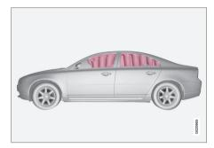
Inflatable curtain IC (Inflatable Curtain) is part of the SIPS system (p. 30) and the airbag system (p. 26). It is fitted in the headlining along both sides of the roof and protects the car's occupants sitting in the outer seats. A sufficiently violent collision trips the sensors and the inflatable curtain is inflated.
