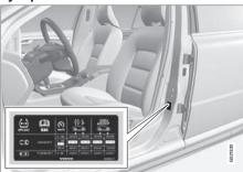
The tyre pressure label on the driver's side door pillar (between frame and rear door) shows which pressures the tyres should have at different loads and speed conditions. This is also specified in the tyre pressure table, see Tyres - approved tyre pressures (p. 387).
