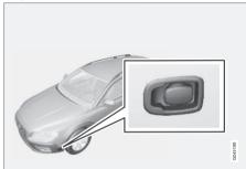
Electrical input to the engine block heater.
