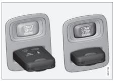
Ignition switch with remote control key extracted/inserted.
