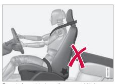
Do not place objects on the rear seat that may prevent the WHIPS system from functioning.
