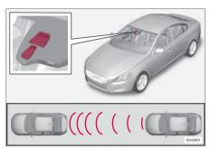
Laser sensor transmitter and receiver window<sup>13</sup>.
