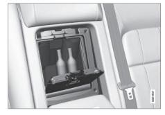
There is a cooler box behind the armrest in the rear seat. The cooler box works when the engine is running or the remote control key is in position II.
