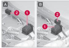
A: Left-hand drive car. B: Right-hand drive car. (1) Starter battery<sup>12</sup> (2) Support battery.
