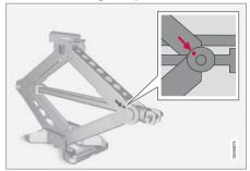
The tools and jack\* must be returned to their correct places after use. The jack needs to be cranked together to the correct position in order to have space.
