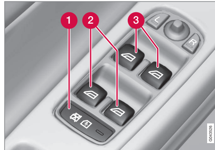
Driver's door control panel.
