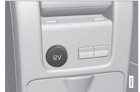
12 V socket in tunnel console, rear seat.
