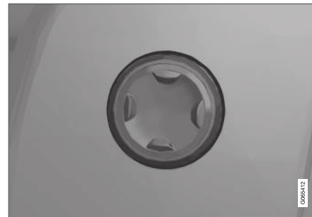
Four-way button, located on the side of the seat's seating section.
