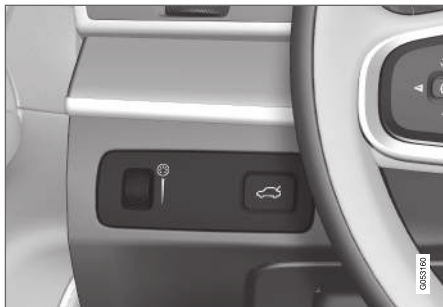
Thumbwheel (to left) for adjusting interior brightness.
