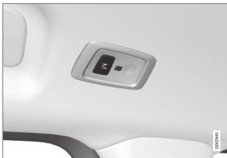
In cars with panorama roof* there are two lamp units, one on each side of the roof.
