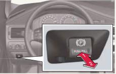
Engage a gear and drive away. The parking brake disengages automatically.
