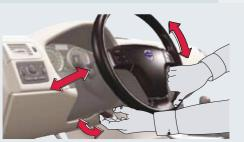
**WARNING!** Adjust the steering wheel before setting off, never while driving.
