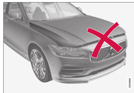
Bonnet not completely closed.
