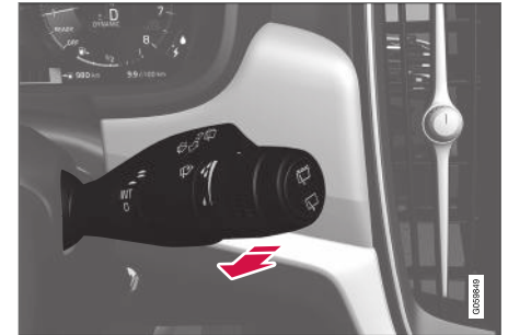
Washing function, right-hand stalk switch.
