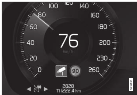
Speed camera information in the instrument panel 99 .
