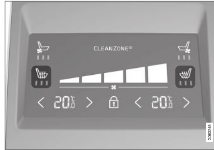
Seat heating controls and indicator lights on the rear side of the tunnel console.
