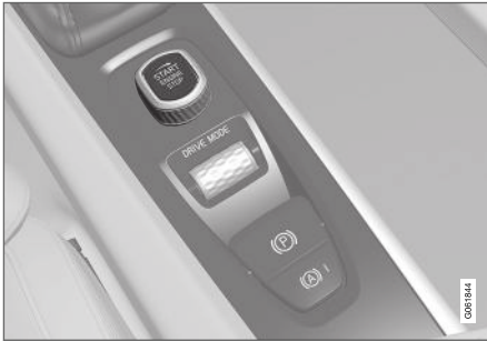
Start knob in the tunnel console.
