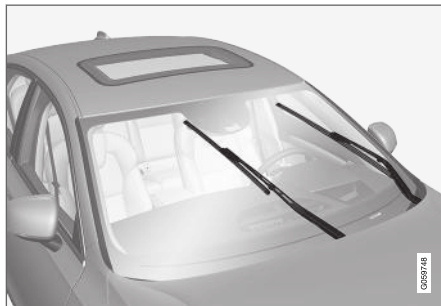
Windshield wipers in the service position.
