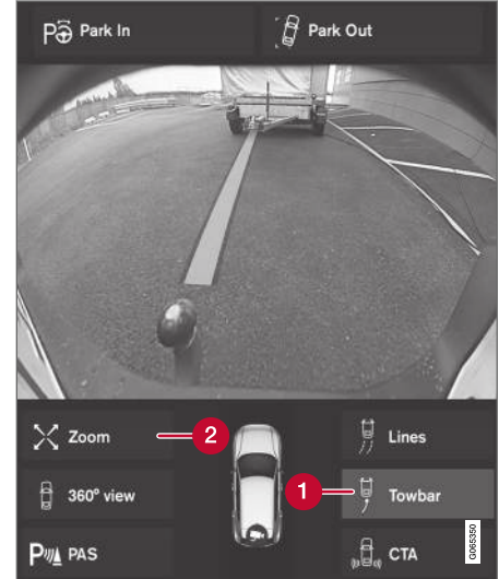
Towbar with trajectory line 117 .
