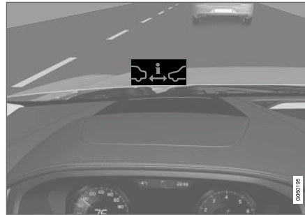
Distance Alert warning symbol on the windshield 33 .
