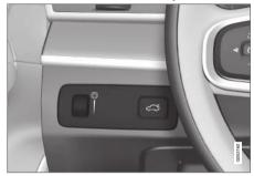
Thumbwheel (to left) for adjusting interior brightness.
