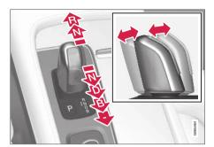
Change gear position by pressing the spring-loaded gear selector forwards or backwards.
