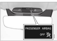
> A text message and a symbol in the roof console indicate that the airbag for the front passenger seat is deactivated.
