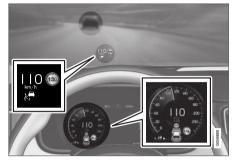
The previous illustration shows that the adaptive cruise control is set to maintain 110 km/h (68 mph) and at the same time is following a vehicle ahead which is keeping the same speed.
