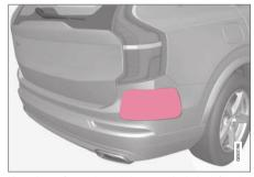
Keep the surface indicated clean – on both the left and right-hand sides of the  $\mbox{car}^{74}$ .
