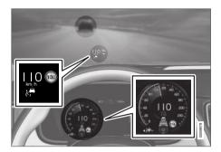
The previous illustration<sup>50</sup> shows that Pilot Assist is set to maintain 110 km/h (68 mph) and at the same time is following a vehicle ahead which is keeping the same speed.
