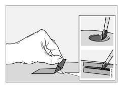
Apply a piece of masking tape over the damaged surface. Then remove the tape to remove any loose paint.
