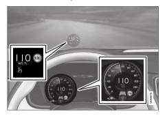
The previous illustration<sup>50</sup> shows that Pilot Assist is set to maintain 110 km/h (68 mph) and that there is no vehicle ahead to follow.
