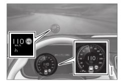
The previous illustration shows that the adaptive cruise control is set to maintain 110 km/h (68 mph) and that there is no vehicle ahead to follow.
