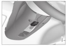
Lever for steering wheel adjustment.
