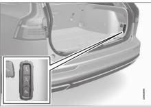
To facilitate folding of the rear seat, the car must be stationary and the tailgate open. Ensure that there are no occupants or objects in the rear seat.
