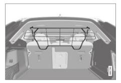
For safety reasons, the safety grille must always be attached and anchored correctly.
