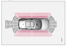
The warning signal pulses intensively at less than approx. 25 cm (0.8 ft) from an obstacle.
