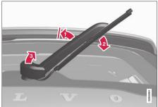
Lift the wiper arm from the windscreen and pull the upper section of the blade diagonally down to the right.
