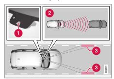
The camera and radar unit measures the distance to the vehicle ahead and detects side markings.
