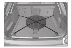
The spare wheel is stored in a bag and must be secured with two straps on the floor of the cargo area while driving. The straps must be tensioned crosswise over the wheel and attached in the car's four load retaining eyelets.
