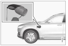
Charging cable handle and charging input socket.
