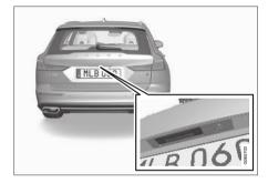
The tailgate is held closed by an electrical lock. To open:
