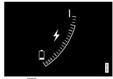
The symbol  $\frac{1}{2}$  is shown in the hybrid battery gauge when Charge is activated.
