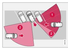
In an angled parking slot CTA may be completely "blind" on one side.
