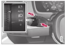
Steering wheel stalk switch with rotating ring.
