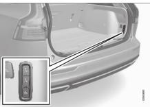
Open the tailgate. A button for extending/ retracting the towbar is located on the righthand side at the rear of the cargo area. An indicator lamp in the button must illuminate with a constant orange glow for the extension function to be active.  Press and release the button – extension might not start if the button is pressed for too long.
