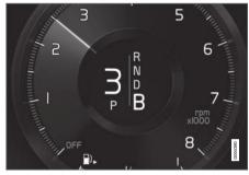
From **B** position, it is possible to gear down manually to lower gears. The **B** position can be selected at any time during travel. The car brakes using its electric motor when the accelerator pedal is released, while also charging the hybrid battery. This gives more opportunities for recharging the hybrid battery, since charging also takes place without the driver using the brake pedal.
