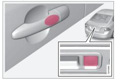
Models with keyless drive have a pressure-sensitive area on the outside door handles and a rubber-covered button next to the trunk opening control
