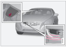
Camera and radar sensor<sup>6</sup>.
