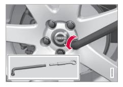
With the vehicle still on the ground, remove the plastic covers on the wheel nuts with the tool provided and use the lug wrench/towing eyelet to loosen the wheel nuts ½ – 1 turn by exerting downward (counterclockwise) pressure.
