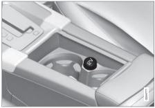
12-volt socket in the front tunnel console
