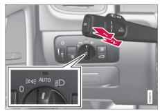
Headlight switch and steering wheel lever
