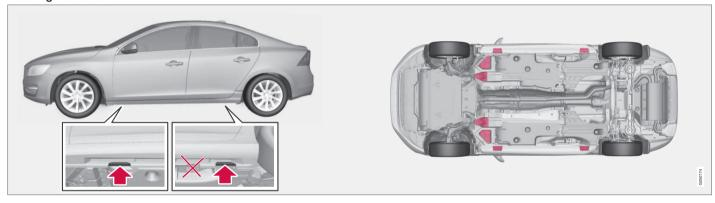
If a garage jack is used to lift the vehicle, it should be placed:
