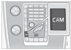
PAC is activated when the gear selector is moved to **R** if the system is selected in the **MY CAR** menu system or by pressing the **CAM** button in the center console. See My Car – introduction (p. 70) for a description of the menu system.
