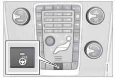
Button for steering wheel heating
