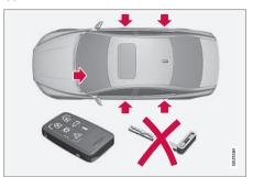
Locking/unlocking points with valet locking activated
