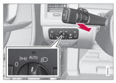
Models with an analog instrument panel When AHB is activated, the symbol will illuminate in the instrument panel. The high beam indicator ( D ) in the instrument panel will also illuminate when the high beams are on.
