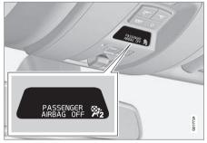
Occupant Weight Sensor (OWS) indicator light
