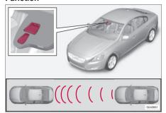
Location of the laser sensor in the windshield<sup>5</sup>
