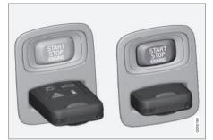
Ignition slot with remote key inserted (see Ignition modes (p. 73) for more information on ignition modes)
