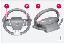
Steering-wheel mounted gear shift paddles
