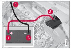
Connecting the jumper cables
