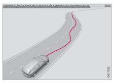
A camera monitors the painted lines marking the lane in which the vehicle is traveling and compares the direction of the road with the driver's movements of the steering wheel. The driver is alerted if the vehicle does not follow the lane smoothly.
