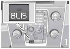
BLIS is automatically activated when the ignition is switched on. The indicator lights will provide confirmation by flashing 3 times.
