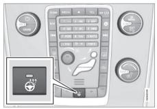
Button for steering wheel heating
