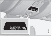
Occupant Weight Sensor (OWS) indicator light
