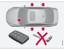
Locking/unlocking points with valet locking activated
