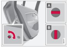
Child safety locks – rear doors The controls are located on the rear door jambs. Use the remote control's key blade or a screwdriver to adjust these controls.
