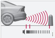
The distance monitored behind the vehicle is approximately 5 ft (1.5 m). The audible signal comes from the rear speakers.
