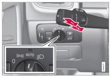
Headlight switch and steering wheel lever
