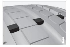
The letters **TWI** are printed on the side of the tire. When approximately 1/16" (1.6 mm) is left on the tread, these strips become visible and indicate that the tire should be replaced. Tires with less than 1/16" (1.6 mm) tread offer very poor traction.
