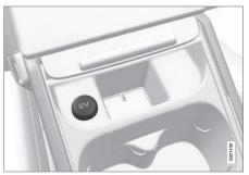
12-volt socket in the front tunnel console
