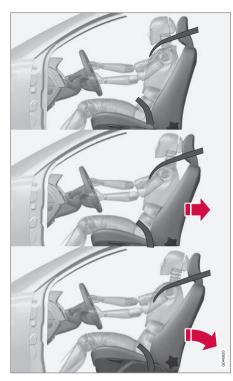
In the event of a rear-end collision, the hinges and brackets of the front seat backrests are designed to change position slightly to allow the backrest/head restraint to help support the occupant's head before moving slightly
