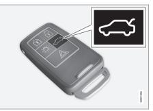
Trunk unlock button on the remote key
