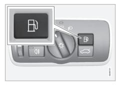
With the ignition switched off, press and release the button on the lighting panel to unlock the fuel filler door. Please note that the fuel filler door will remain unlocked until the vehicle begins to move forward. An audible click will be heard when the fuel filler door relocks.
