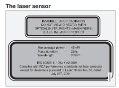
The upper decal describes the laser beam's classification and contains the following text:
