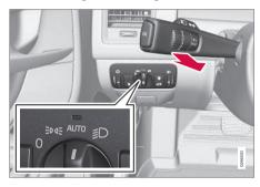
**Models with an analog instrument panel** When AHB is activated, the Symbol will illuminate in the instrument panel. The high beam indicator (S) in the instrument panel will also illuminate when the high beams are on.
