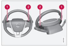
Steering-wheel mounted gear shift paddles
