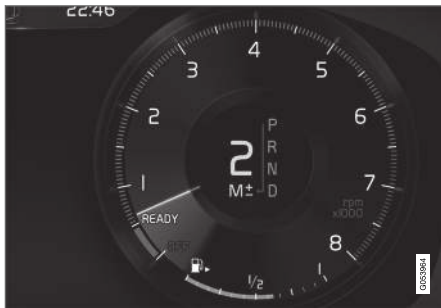
manual gearshift mode in the driver display 3 .
