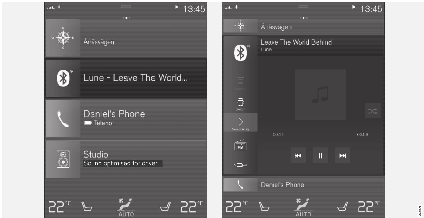
Standard mode and expanded mode of a tile in the centre display.
