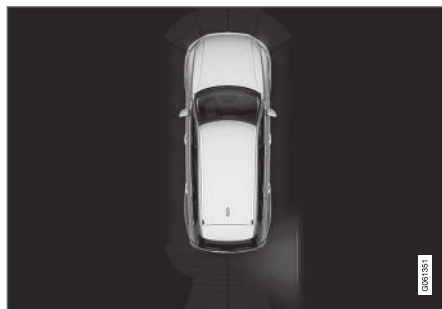
Illuminated icon for CTA in the PAS 87 graphic on the screen 88 .
