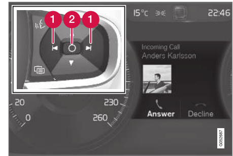
Message in the driver display 7 and the steering wheel's right-hand keypad.
