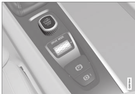
Start knob in the tunnel console.
