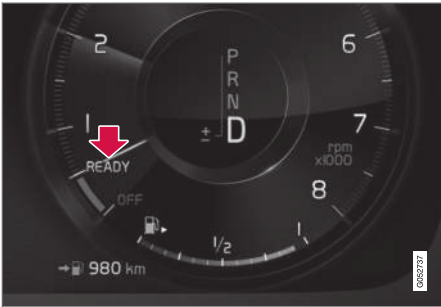
The function is active and the engine is auto-stopped.
