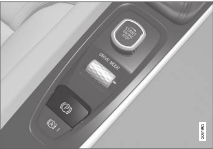
The control for the parking brake is located in the tunnel console between the seats.
