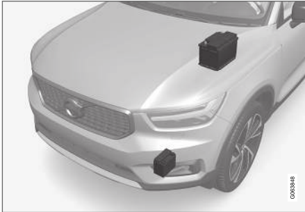
The support battery is located down in the engine compartment. The starter battery is also shown here (top).
