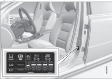
The tyre pressure label on the driver's side door pillar (between frame and rear door) shows which pressures the tyres should have at different loads and speed conditions. This is also specified in the tyre pressure table, see Tyres - approved tyre pressures (p. 427).
