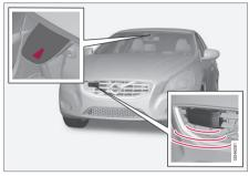
Camera and radar sensor<sup>21</sup>.
