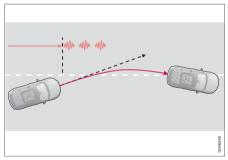
Warning with steering wheel vibration<sup>27</sup>.
