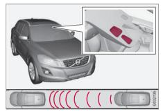
Laser sensor transmitter and receiver window13.
