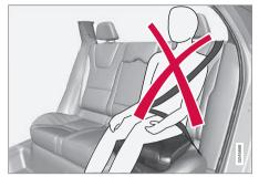
Incorrect positioning, the seatbelt must not be placed heneath the shoulder
