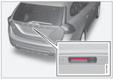
Rubber plate with electrical contact.
