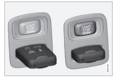
Ignition switch with remote control key extracted/inserted.
