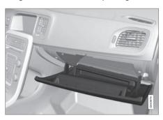
The owner's manual and maps can be kept in here for example. There are also holders for pens on the inside of the lid. The glovebox can be locked\* (p. 181) using the key blade (p. 169).
