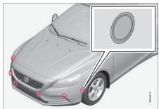
The PAP sensors are located in the bumpers<sup>37</sup> - 6 front and 4 rear.
