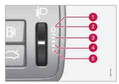
Thumbwheel positions for different load cases.
