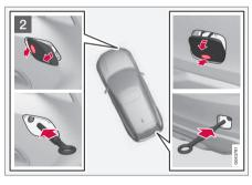
Take out the towing eye that is located under the floor hatch in the cargo area.
