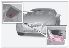
Camera and radar sensor<sup>6</sup>.
