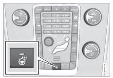
Button for steering wheel heating
