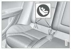
Symbols on the seat back upholstery mark the ISOFIX/LATCH anchor positions as shown. To access the anchors, kneel on the seat cushion and locate the anchors by feel. Always follow your child seat manufacturer's installation instructions, and use both ISOFIX/LATCH lower anchors and top tethers (p. 59) whenever possible.
