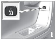
The indicator light in the button is on when the door is locked  $% \left\{ 1,2,\ldots ,n\right\}$
