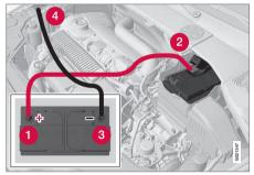
Connecting the jumper cables
