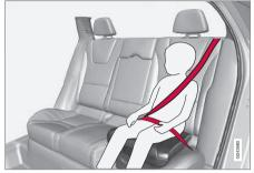
Correct seating position: the shoulder belt is across the collarbone
