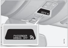
Occupant Weight Sensor (OWS) indicator light
