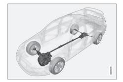
Under normal driving conditions, most of the engine's power is directed to the front wheels. However, if there is any tendency for the front wheels to spin, an electronically controlled coupling distributes power to the wheels that have the best traction.
