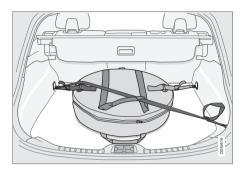
Turn the handle on the spare wheel bag out toward you. Secure the stitched strap hooks in the front loading eyelets. Secure the long strap in one of the front loading eyelets, wrap the strap diagonally over the spare wheel and through the upper handle. Secure the short strap on the long strap. Secure in the rear loading eyelet and tighten.
