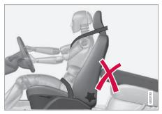
Any contact between the front seat backrests and the folded rear seat or a rear-facing child seat could impede the function of the WHIPS system. If the rear seat is folded down, the occupied front seats must be adjusted forward so that they do not touch the folded rear seat.
