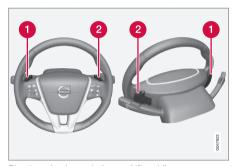
Steering-wheel mounted gear shift paddles
