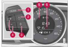
Steering wheel-mounted controls and display
