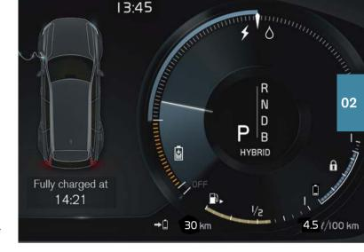
that the hybrid battery is being charged if its charge level is low. **Hold** means that the battery level is being retained for later use.
