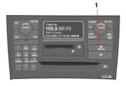
By holding the button depressed you can fast forward or rewind in a song or search for a radio station.
