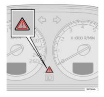
**NOTE!** When the message text "TIME FOR REGULAR SERVICE" is shown, the symbol lamp and message text are cleared using the READ button, or disappear automatically after 2 minutes.
