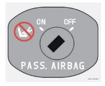
Switch for SRS in ON position.
