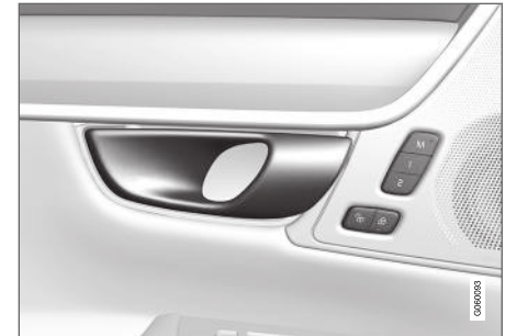
Opening handle for alternative unlocking in the side door 12 .
