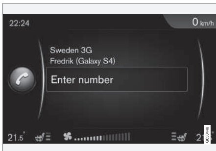
An example of telephone mode's normal view
