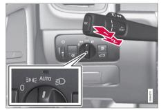
Headlight switch and steering wheel lever
