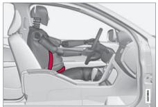
The seat belt should always be worn during pregnancy. But it is crucial that it be worn in the correct way. The diagonal section should wrap over the shoulder then be routed between the breasts and to the side of the belly. The lap section should lay flat over the thighs and as low as possible under the belly. It must never be allowed to ride upward. Remove all slack from the belt and ensure that it fits close to the body without any twists.
