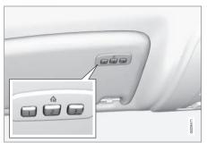
The HomeLink¹ Wireless Control System provides a convenient way to replace up to three hand-held radio-frequency (RF) transmitters used to activate devices such as gate operators, garage door openers, entry door locks, security systems, even home lighting. Additional HomeLink information can be found on the Internet at www.homelink.com or by phoning the hotline at 1–800–355–3515.
