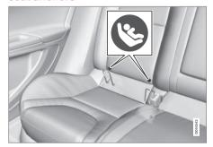
Lower anchors for ISOFIX/LATCH-equipped child seats are located in the rear, outboard seats, hidden below the backrest cushions. Symbols on the seat back upholstery mark the anchor positions as shown. To access the anchors, kneel on the seat cushion and locate the anchors by feel. Always follow your child seat manufacturer's installation instructions. and use both ISOFIX/LATCH lower anchors and top tethers whenever possible.
