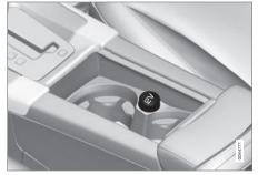
12-volt socket in the front tunnel console
