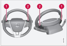
Steering-wheel mounted gear shift paddles
