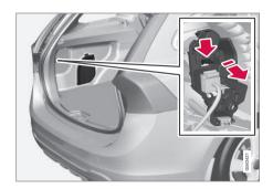
The backup lights, fog lights and turn signals are replaced from inside the cargo area
