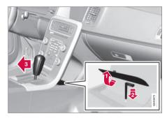
If the vehicle cannot be driven, for example because of a dead battery, the gear selector must be moved from the **P** position before the vehicle can be moved<sup>4</sup>.
