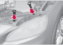
Plug in the connector until it clicks into place.  Reinstall the headlight housing and locking pins. The short locking pin should be closest to the grille. Check that they are correctly inserted.
