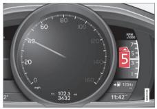
Gear shift indicator in a digital instrument panel\*2
