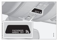
Occupant Weight Sensor (OWS) indicator light
