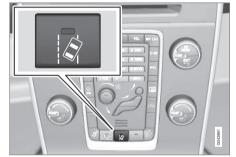
LDW can be switched on or off by pressing the button on the center console. A light in the button illuminates when the function is on. This is supplemented by graphic displays in the instrument panel, for example:
