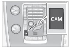
PAC is activated when the gear selector is moved to **R** if the system is selected in the **MY CAR** menu system or by pressing the **CAM** button in the center console. See page 219 for a description of the menu system.
