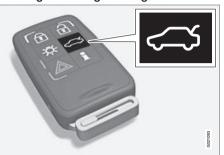
Tailgate unlock button on the remote key
