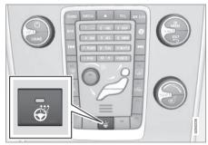
Button for steering wheel heating
