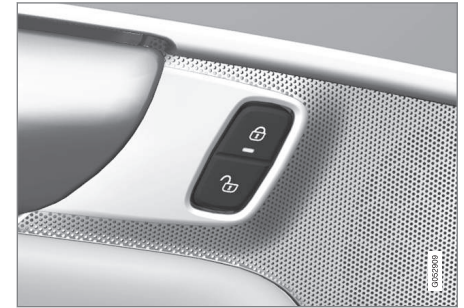
Front door lock button and indicator light
