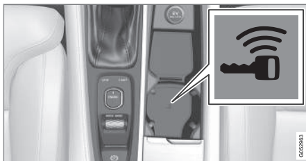
Back-up reader in the tunnel console
