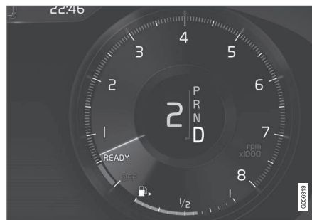
Instrument panel when the paddles are activated
