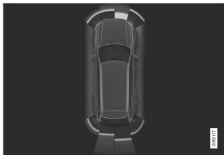
Display view showing object zones and sensor sectors
