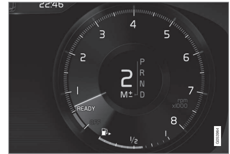
Manual shift indicator in the instrument panel 5 .
